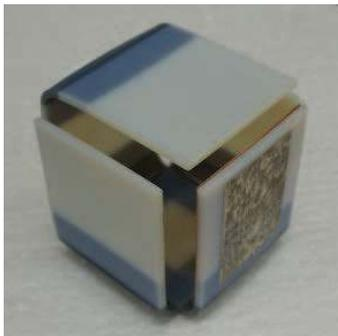
Fig. 21. A flexible 3D printed SMA cube with an inkjet-printed antenna on one of its faces
