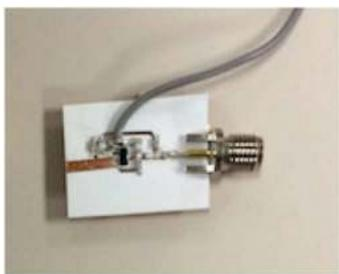
Fig. 31. Inkjet-printed flexible reflection amplifier prototype.
